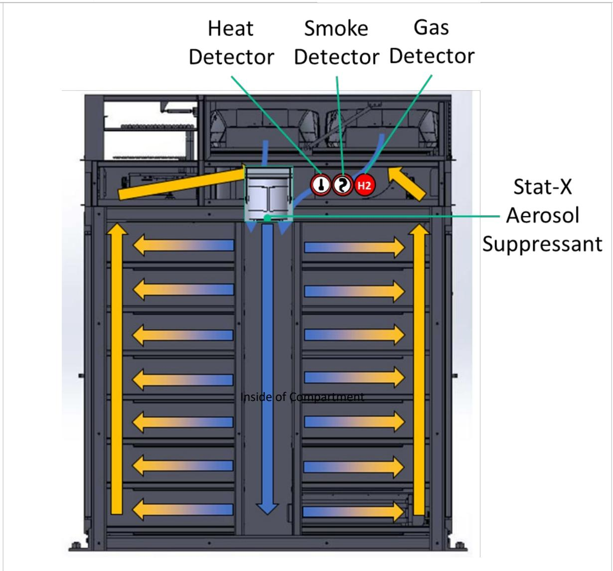
**Figure 4.** Stat-X Fire Suppression System Device Layout
