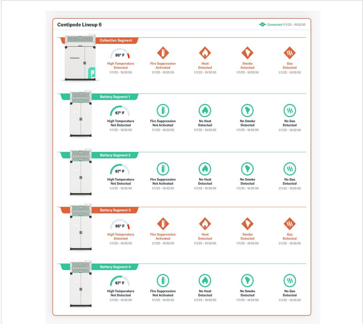
Figure 5. Stack750E Status Page of the Powin for First Responders HMI
